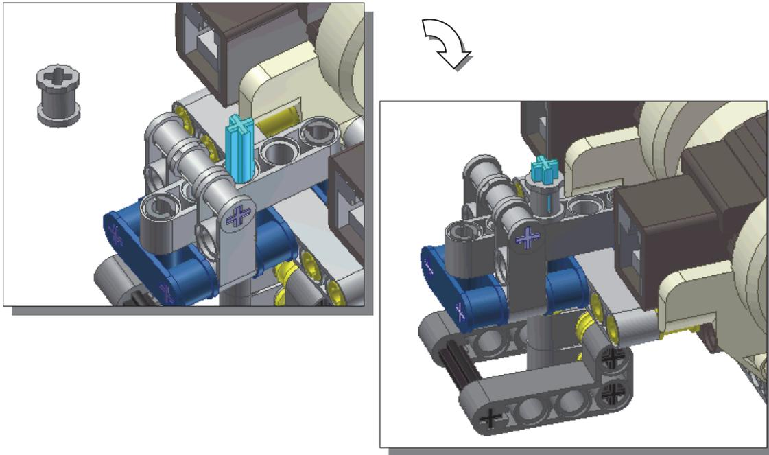
24. On your own, assemble a **Wheel-Small** assembly and two copies of the **Wheel 56x26 VR** assembly as shown.
