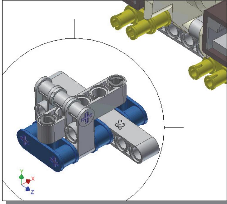
11. On your own, apply the necessary constraints to align the subassembly to the two **Peg 2-module Double** parts as shown.
