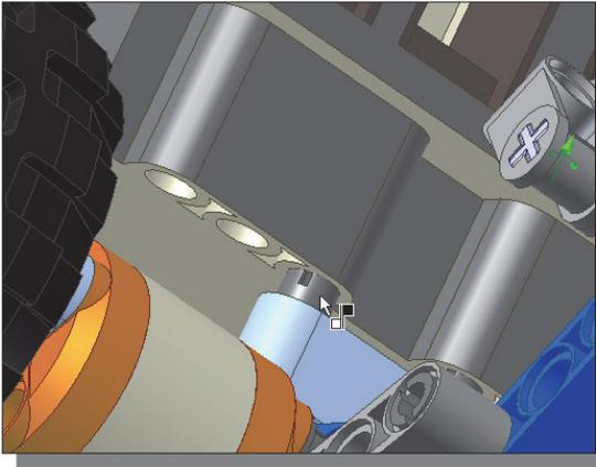
9. Select the outside cylindrical surface of the left **Peg 1-Module** part of the **Frame-Front** assembly as shown.
