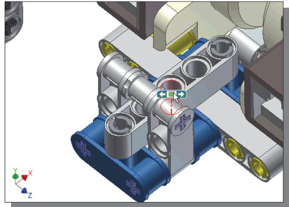
18. Select the curved surface of the **Axle** part of the **Rear-Swivel** assembly as the 2<sup>nd</sup> item for the **Constrain** command.
