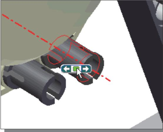
9. Select the circular face of the back **Peg** part of the **Motor-Left** assembly as the 2<sup>nd</sup> item for the **Constrain** command.
