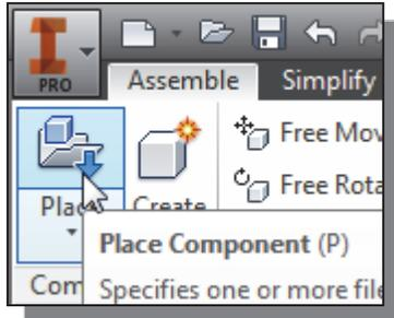
13. In the *Assemble* panel, select the **Place Component** command by left-mouse-clicking once on the icon.
