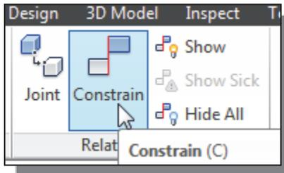
3. In the *Position* panel, select the **Constrain** command by left-mouse-clicking the icon. On your own, assemble the three parts as shown in the figure.
