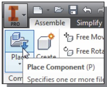
12. In the *Assembly* panel, select the **Place Component** command by left-mouse-clicking the icon.
