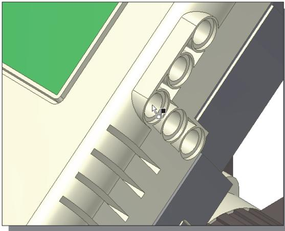
7. On your own, align the center axes of the lower **Peg** on the **Arm** assembly to the corresponding hole feature on the **NXT-Brick** assembly. (The top of the **Beam 9-module** part on the **Arm** assembly is parallel to the top of the **NXT-Brick**.)
