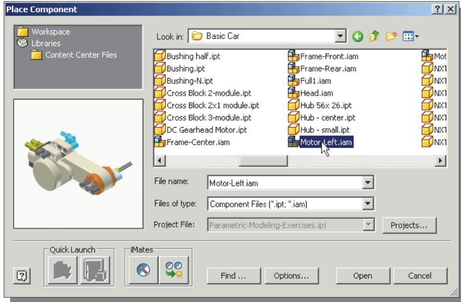
3. Place a copy of the **Motor-Left** assembly to the left side of graphics area.
