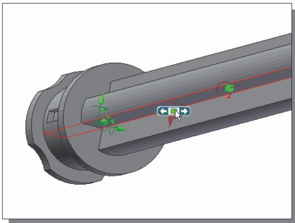
8. Select the corresponding **flat surface** of the *Axle-8* part as shown.
