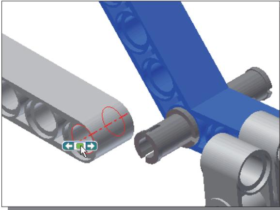
6. Select the first hole feature, on the inside cylindrical surface, of the left **Beam 13-module** as shown.
