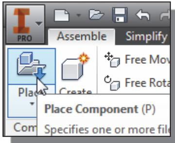
5. In the *Assembly* panel, select the **Place Component** command by left-mouse-clicking the icon.
