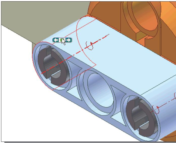
24. On your own, align the center axis of the left feature to the center axis of the other *Peg 1-Module* part as shown.
