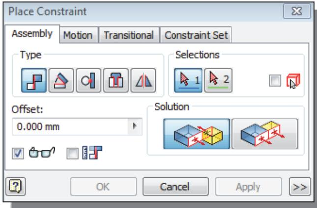
7. In the *Place Constraint* dialog box, confirm the constraint *Type* is set to the **Mate** constraint.
