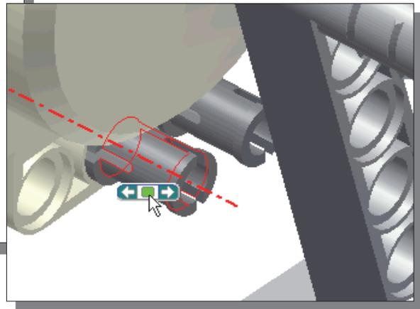
12. Also apply a **Mate** constraint to align the inside surface of the **Motor** subassembly as shown.
