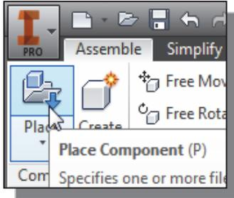
18. In the *Assembly* panel, select the **Place Component** command by left-mouse-clicking the icon.
