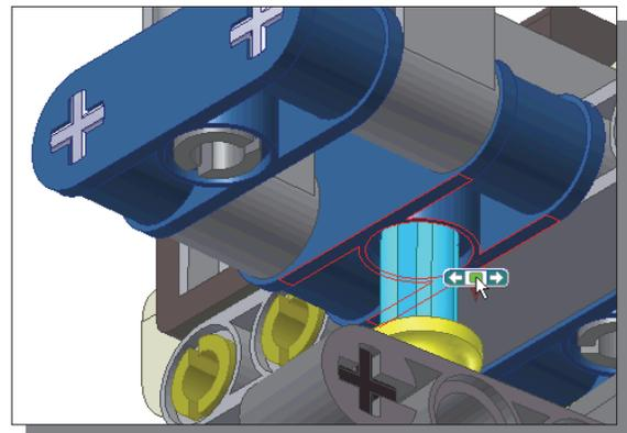
21. Select the top surface of the **Bushing** part of the **Rear-Swivel** assembly as the 2<sup>nd</sup> item for the **Constrain** command.
