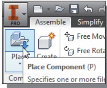
1. In the *Assembly* panel, select the **Place Component** command by left-mouse-clicking the icon.
