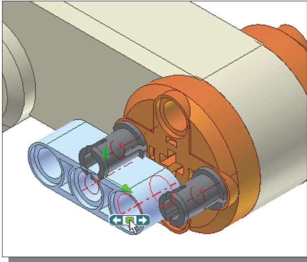
21. Select the **right inside cylindrical surface** of the *Beam 3-Module* component, the chassis rail, as the first item for the **Mate Alignment** command.
