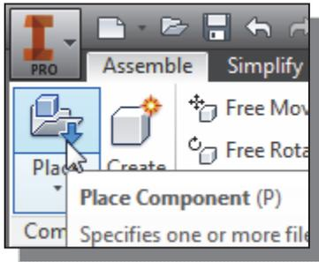
9. In the *Assembly* panel, select the **Place Component** command by left-mouse-clicking once on the icon.
