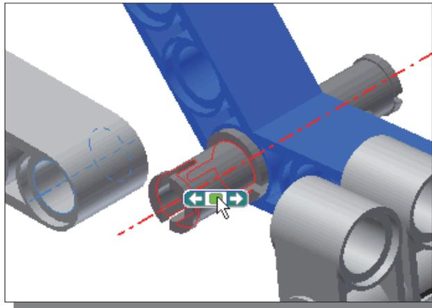
9. On your own, repeat the above steps and assemble the **Frame-Center** subassembly and the other **Beam 13-module** as shown.
