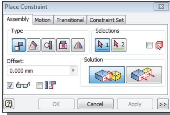
6. In the *Place Constraint* dialog box, set the constraint *Type* to the **Mate** constraint.
