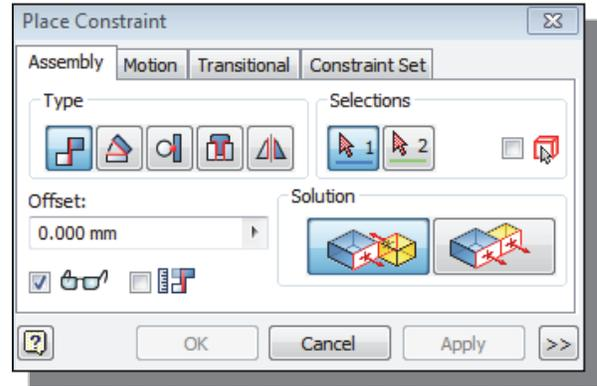
2. In the *Place Constraint* dialog box, switch to the **Mate** constraint.
