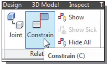
7. In the *Assembly* panel, select the **Constrain** command by left-mouse-clicking once on the icon.
