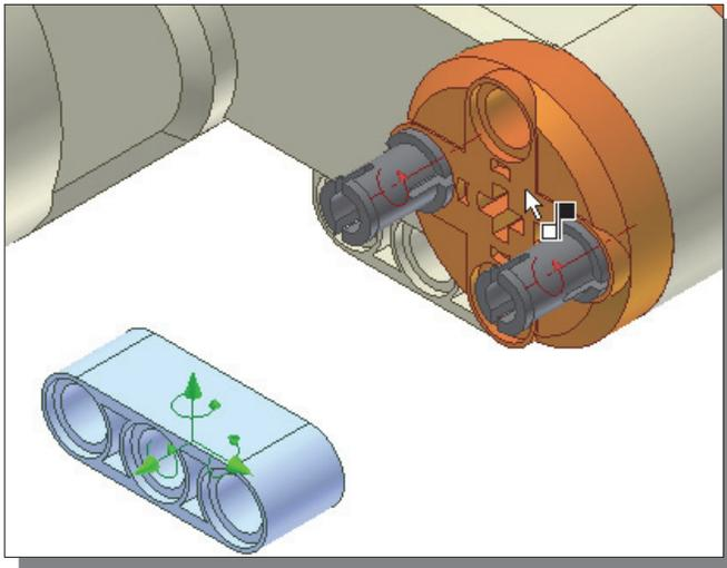
18. Select the **front vertical surface** of the base component, the chassis rail, as the first item for the **Mate Alignment** command.
