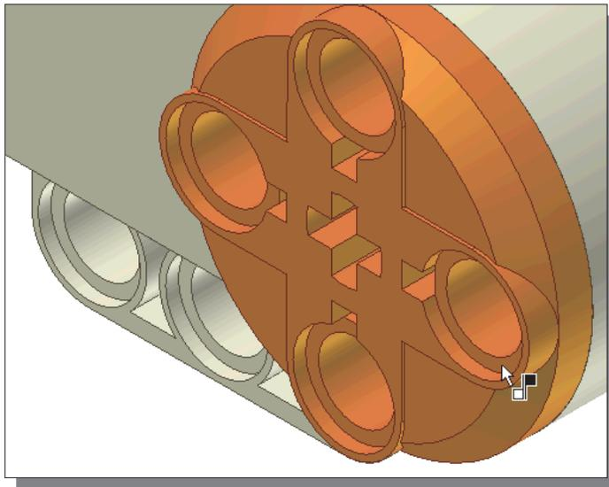
3. Select the ring surface of the **NXT Motor Drive** as the first item for the **Mate Alignment** command.
