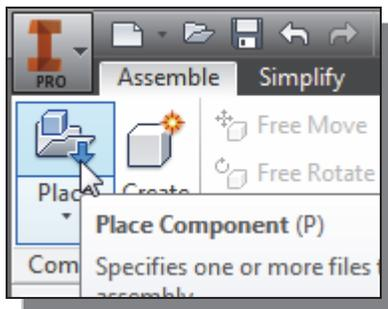
1. Switch to the *Assembly* panel, and select the **Place Component** command by left-mouse-clicking the icon.
