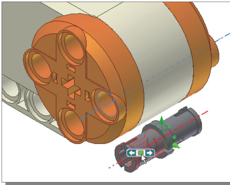
9. Click on one of the **outside cylindrical surfaces** of the **Peg 1-Module** part as the second item to apply the constraint.
