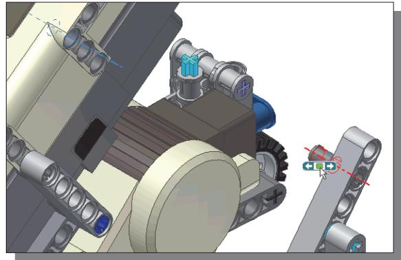
6. Align the center axes of the upper **Peg** on the **Arm** assembly to the corresponding hole feature on the **NXT-Brick** assembly as shown in the two figures.
