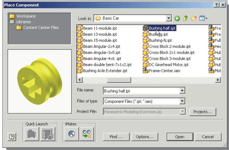
2. Select the **Bushing half** design in the list window. Click on the **Open** button to retrieve the model.
