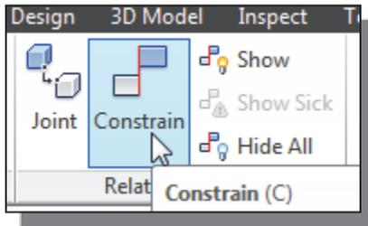
1. In the *Assembly* panel, select the **Constrain** command by left-mouse-clicking once on the icon.
