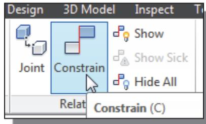
5. In the *Assembly* panel, select the **Constrain** command by left-mouse-clicking once on the icon.
