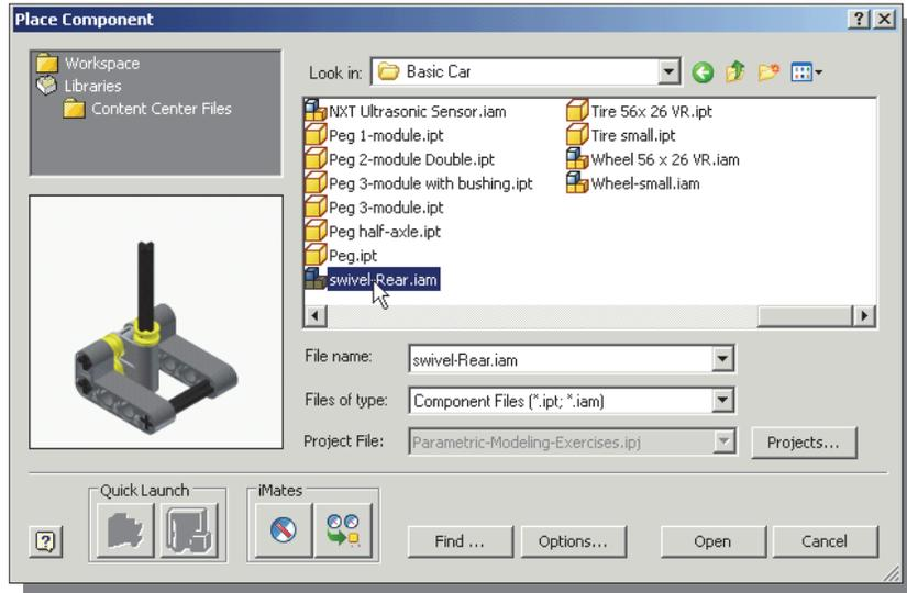
14. Place one copy of the **Swivel-Rear** assembly next to the assembly.
