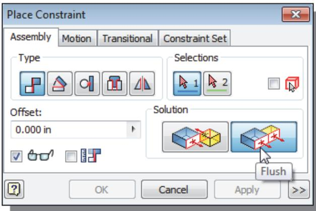
4. In the *Place Constraint* dialog box, set the constraint *Type* to the **Flush** constraint.
