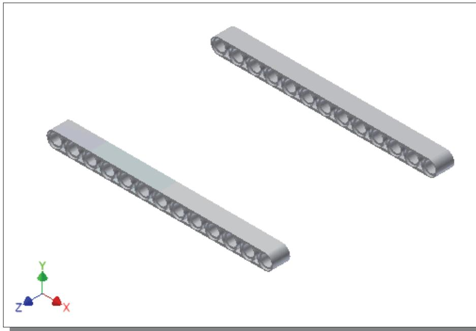
12. Inside the graphics window, right-mouse-click once to bring up the option menu and select **Done** to end the placement of the **Beam 13-module** parts.
