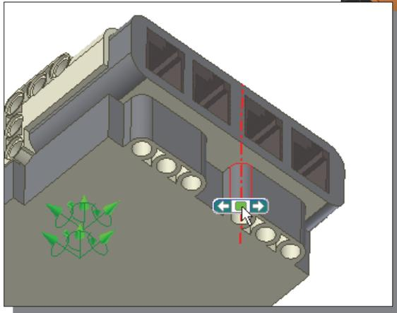
7. Select the center axis of the first hole feature on the bottom right of the **NXT-Brick** assembly as shown.
