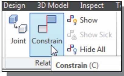
16. In the *Assembly* panel, select the **Constrain** command by left-mouse-clicking once on the icon.
