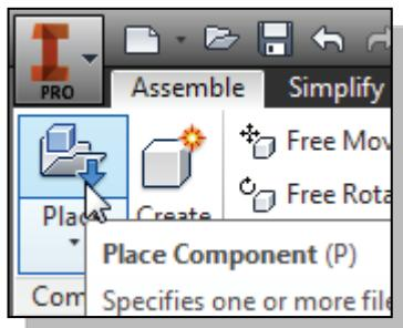
13. In the **Assembly** panel, select the **Place Component** command by left-clicking once on the icon.
