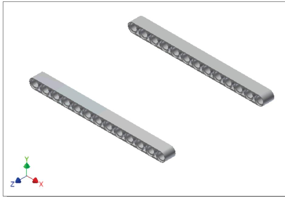
12. Inside the graphics window, right-click once to bring up the option menu and select **Done** to end the placement of the **Beam 13-module** parts.
