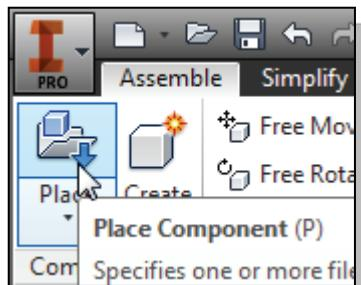
7. In the *Assembly* panel, select the **Place Component** command by left-clicking the icon.
