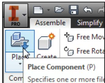
1. In the *Assembly* panel, select the **Place Component** command by left-mouse-clicking the icon.
