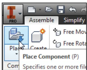
10. In the *Assembly* panel, select the **Place Component** command by left-mouse-clicking the icon.
